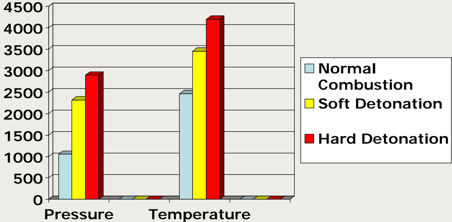
**No OEM Combustion Chamber is designed to handle the types of pressures and temperatures that are caused by detonation.**
