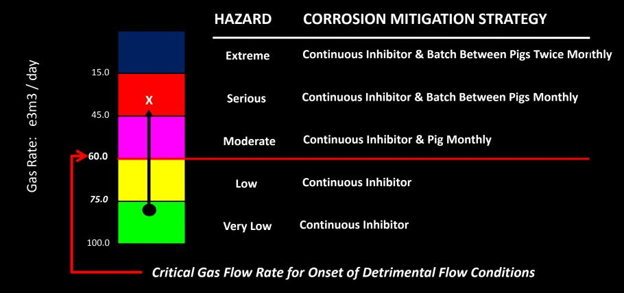
Implication of changing conditions can be identified by Field, Operations and corrective action taken to reduce likelihood of IC corrosion failure event
