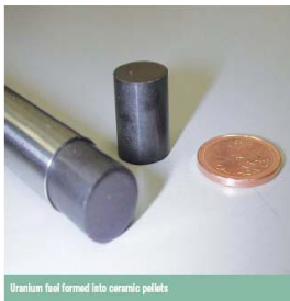
Uranium fuel formed into ceramic pellets
